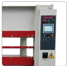
Control Panel / PLC Interface
