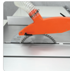
Cutting Unit, Guard Assembly
