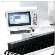
HMI Operator Station
