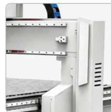
Gantry Side Support and Precision Linear Rails
