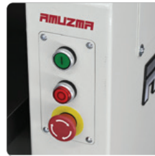
Main Control Panel with Emergency Stop
