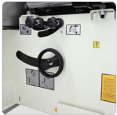
Blade Tilt and Height Adjustment Controls
