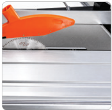
Overhead Saw Blade Guard (Crown Guard)
