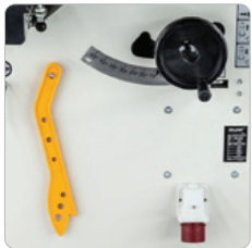
Spindle Tilt Handwheel and Angle Scale
