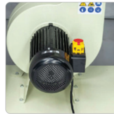
Induction Motor with Magnetic Safety Switch
