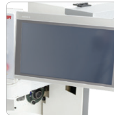
PLC Touchscreen Control Panel
