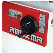
Spindle Height Handwheel and Main Control Panel
