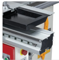
Sliding Table with End with Tool Tray
