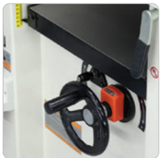
Manual Handwheel with Readout
