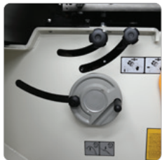
Scoring Blade Adjustment Controls
