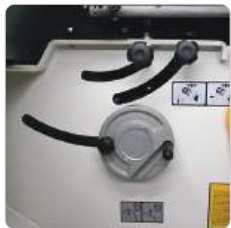
Scoring Blade Adjustment Controls
