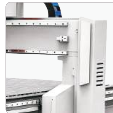
Gantry Side Support and Precision Linear Rails
