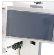
PLC Touchscreen Control Panel
