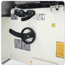
Blade Tilt and Height Adjustment Controls
