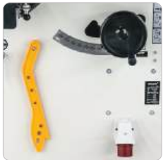
Spindle Tilt Handwheel and Angle Scale
