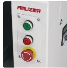
Main Control Panel with Emergency Stop
