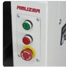
Main Control Panel with Emergency Stop
