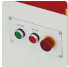
Main Control Panel with Emergency Stop
