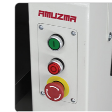
Main Control Panel with Emergency Stop
