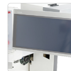
PLC Touchscreen Control Panel
