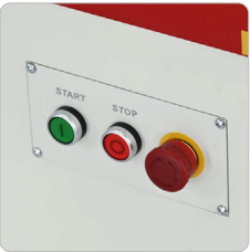
Main Control Panel with Emergency Stop
