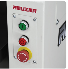
Main Control Panel with Emergency Stop
